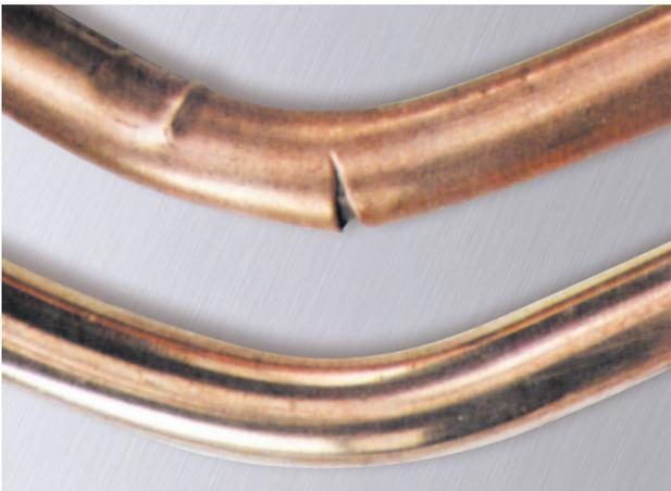
**Figure 76.** Copper bonded and copper clad earth rods.
